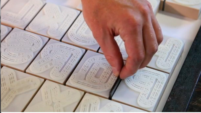
New North Press attempts to use 3D printing to find new possibility in the industry of letterpress.
